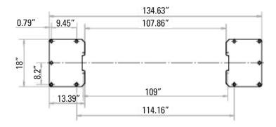
**STEP 8**: Use the existing holes in column base plate as a guide for drilling the 3/4" diameter holes into the concrete. Drill the anchor holes only for ONE column, installing anchors as you go. You will install anchors in second column after the cables, hoses, and floorplate are installed.
