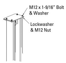
**STEP 7**: Position the columns facing each other **134-5/8**" outside base plates. Square the columns by measuring diagonally from corner points on base plates (within 1/4").
