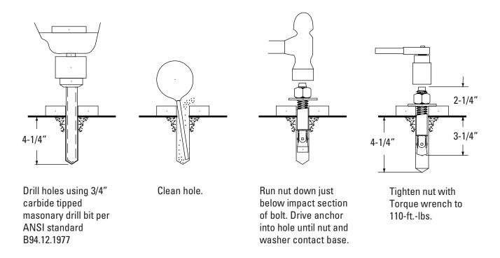
**STEP 9**: Using a level, check column for side-to-side plumb and front-to-back plumb. If needed, use horseshoe shims provided by placing shims underneath the base plate and around the anchor bolt. This will prevent bending the column bottom plates (Shim thickness should not exceed 1/2"). Tighten 3/4" anchor bolts to **110 ft-lbs.** of torque.
