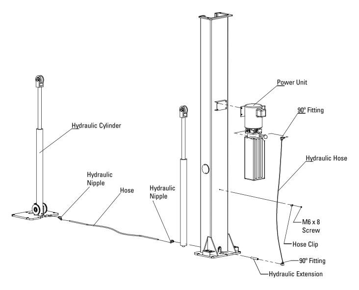
STEP 15: Mount the Power Unit on lift as shown.
