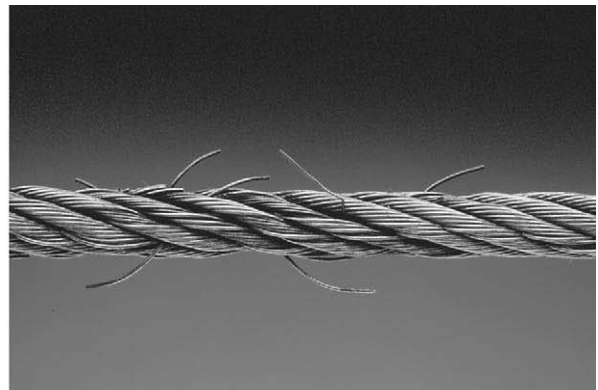
Cable With Broken Wires
