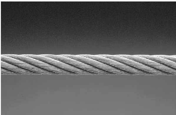
Typical Good Cable
